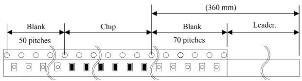
Material of carrier tape : Polyst Material of cover tape : Polyest
